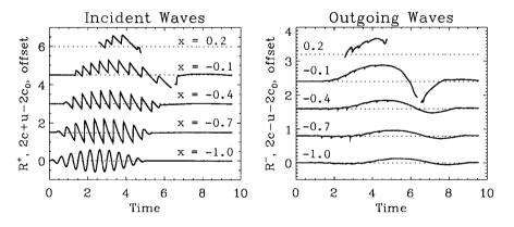
Figure 3: Plots of incident and outgoing wave signals (Riemann Invariants) at various distances offshore, for the waves in figure 2.
