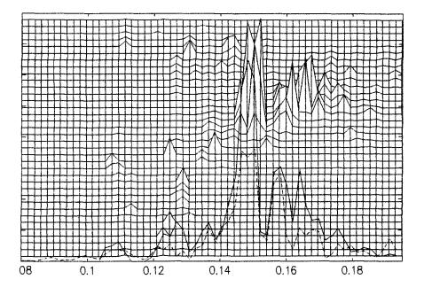
Fig. 9 3D plot of directional spectrum (frontal view). Vertical axis is direction and horizontal axis is frequency (axis z is spectral density). In the same graph one point spectrum.
