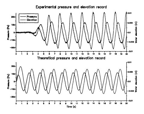
Figure 4: Air pressure and water elevation results, f=0.5Hz, wave amplitude=10mm, orifice=10x10mm
