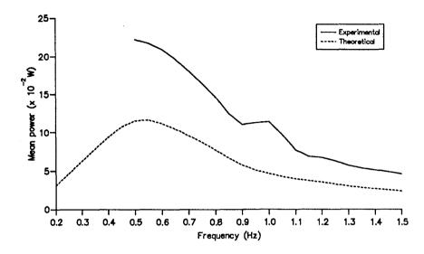
Figure 5: Calculated instantaneous power, orifice=25x25mm, wave amplitude=10mm
