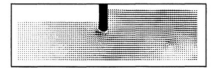
Figure 2: PIV vector map, f=0.6Hz, wave amplitude=15mm
