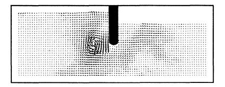
Figure 3: PIV vector map, f=0.6Hz, wave amplitude=15mm
