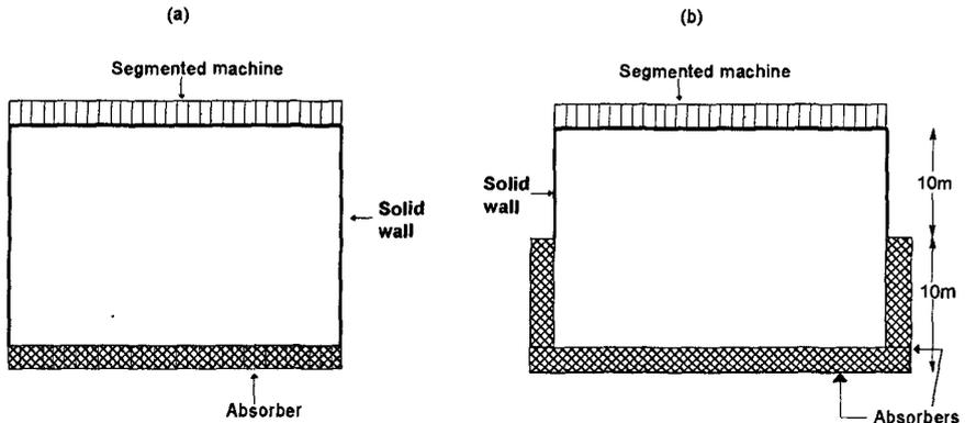
Figure 3: Layout of Basins for Verification of Dalrymple's Theory
