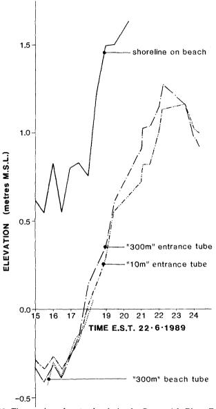
**Figure 10**: Time series of water levels in the Brunswick River Entrance (22–6–89) (10m tube and 300m tube) and on the southern beach (shoreline). Offshore RMS wave height increased from 2.4m at 1500hrs to 3.2m at 2400hrs, while wave period averaged 12 seconds.
