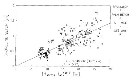
Figure 5: Shoreline setup plotted as a function of wave height  $(H_{orms})$  for all data
