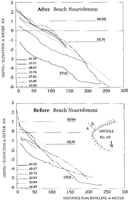
Fig. 6: Beach-Profiles in the groyne-field (A-D<sub>1</sub>)
