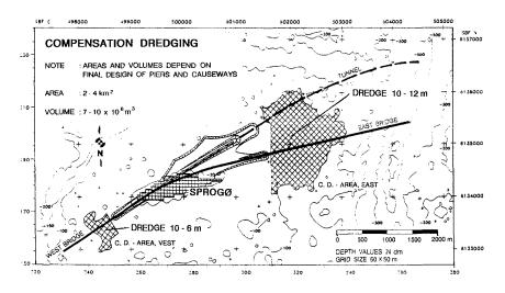
Fig. 2. Typical Compensation Dredging
