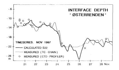
Fig. 9. Time Series of Measured and Calculated Density Interface at Measurement Station 'Østerrende' shown in Figure 8. Note the Rapid Change in Position on Nov. 24. This Change is Associated with the Occurrence of Internal Hydraulic Control of the Two Layer Flow.
