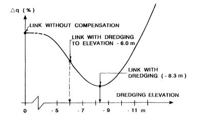
Fig. 4. Water Flow Deviation as a Function of Compensation Dredging Elevation
