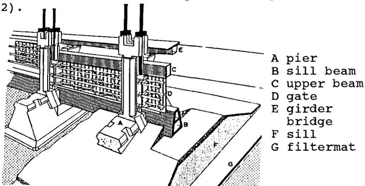
Figure 2: Elements of the Eastern Scheldt Barrier
