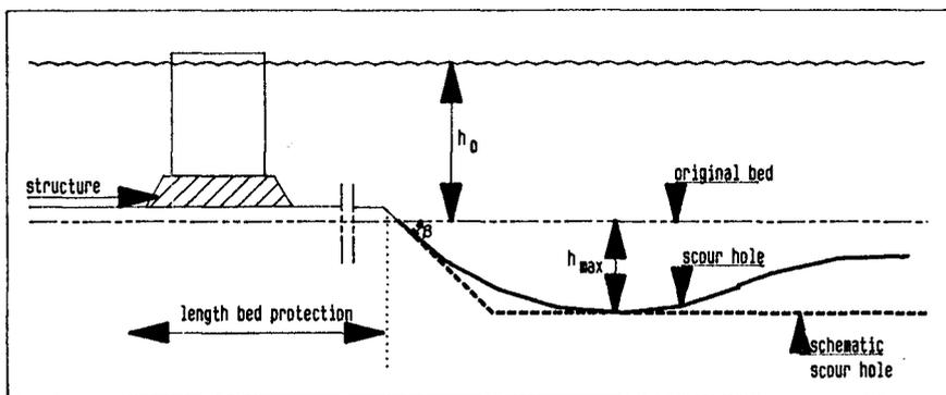
$$t_1 = \frac{330 \cdot \Delta^{1.7} \cdot h_0^2}{(\alpha U - U_{cr})^{4.3}} \quad (1) \quad \text{and} \quad \frac{h_{max}}{h_0} = \frac{t}{t_1}^p \quad (2)$$
