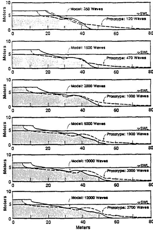
Figure 3: Comparisons between GWK and  $\frac{1}{10}$  Scale Model with  $N_t = N_\lambda = 10$  and  $N_i = 1$  (from Dette and Uliczka, 1986).
