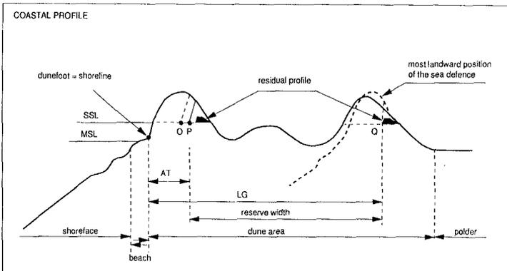
Figure 4 Schematic cross-section of the coastal defence area with definition of the procedure for evaluating problems with flood-protection.
