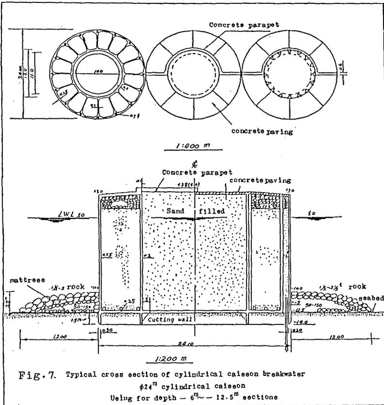
Fig. 7. Typical cross section of cylindrical caisson breakwater
