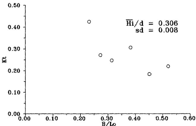
Fig. 10.- A Typical Example of  $K_t$  versus  $B/L_0$ , for  $\bar{H}_i/d=0.306$  (Crest Freeboard  $F=0.00$  m.).
