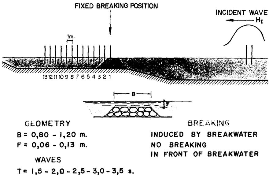
Fig. 7.- Scheme of Transmitted Wave Evolution Model Set-Up.
