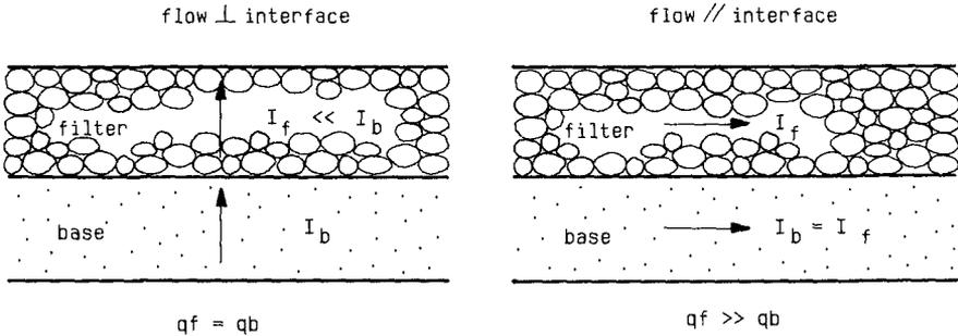
Figure 3 Hydraulic gradients
