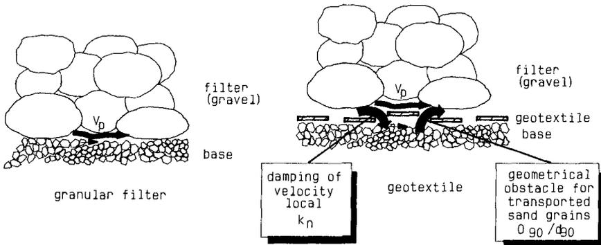
Figure 10 Principle of erosion at interface
