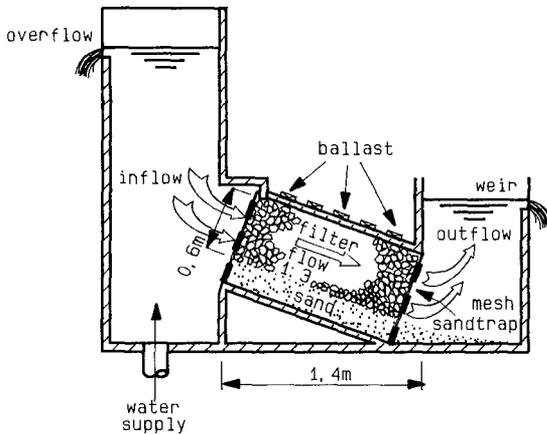
Figure 7 Delft Hydraulics Filter-box, with inclined interface
