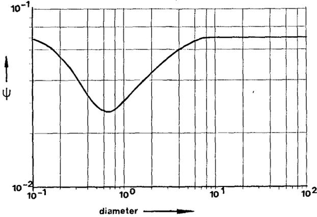
Figure 4 Shields parameter.
