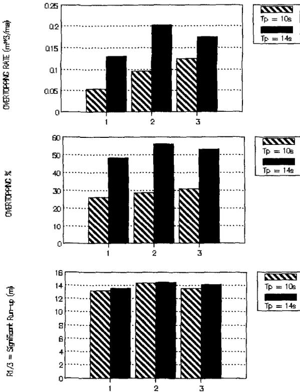
Figure 12. Results from solutions 1,2,3 with  $H_s=7.5m$
