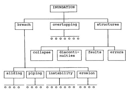
Figure 8: Failure Tree for a Dike-ring
