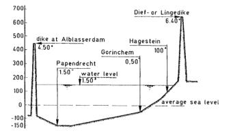
Figure 6: Schematic cross section of Alblasserwaard
