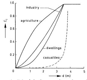
Figure 4: Material loss and number of casualties as a function of the inundation depth (examples)
