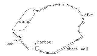
Figure 2: A dike-ring is an area surrounded by a system of water retaining elements as dunes, sheel walls, locks and so on.
