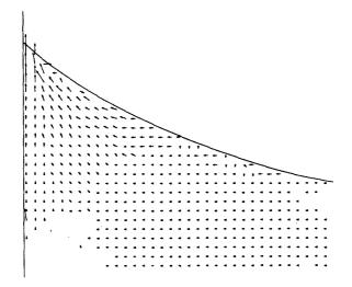
Figure 4. Observed Flow Velocities in a Solitary Wave Running Up on a Vertical Wall
