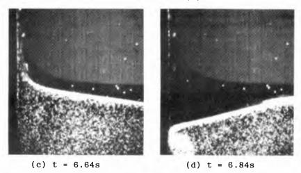
Photo 1. Solitary Wave Runup on a Vertical Wall
