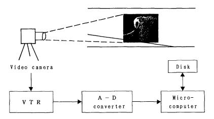
Figure 3. Data Acquisition and Processing System
