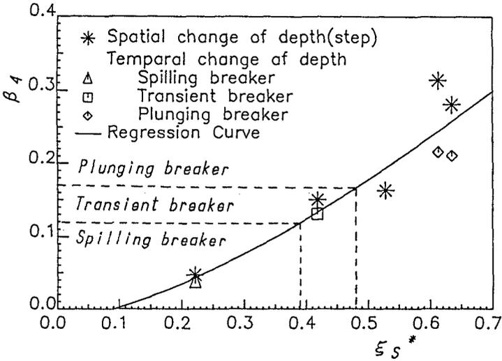
Fig.6 Relation with the breaking of a solitary wave caused by a step between  $\xi_s^*$  and  $\beta_4$
