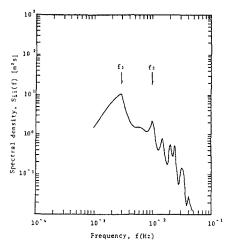
Fig.-11 Low frequency power spectrum of a incident wave groups
