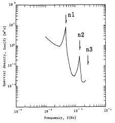
Fig. -10 Power spectrum of the low frequency oscillation of mean sea level at point 3
