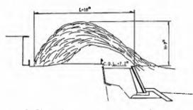
Fig. -2 Sketch of an overtopping wave
