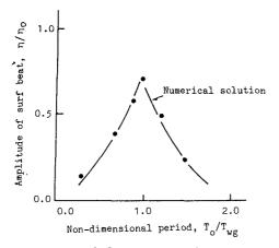
Fig. -8 Resonance diagram (η<sub>o</sub>, Twg :root mean square amplitude and period of incident wave groups )
