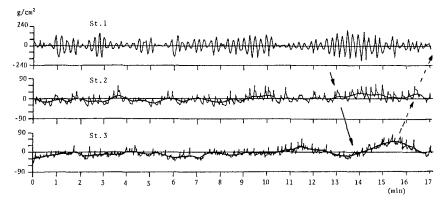
Fig.-9 Wave gage records simultaneously obtained for Typhoon T8520 at three different locations
