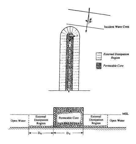
Figure 1: Plan view (upper) and cross-section (lower) of model breakwater.
