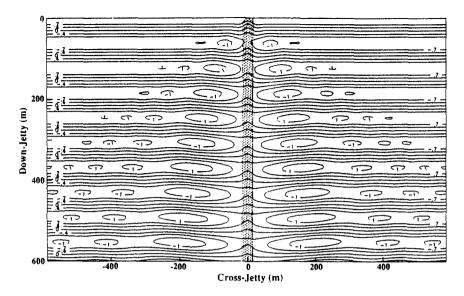
Figure 2: Normalized, instantaneous surface elevation field. Incoming wave: incidence angle = 0°, period = 14 sec, height = 0.8 m, lenght = 120 m. Model jetty: core width = 32 m, stone diam. = 1.25 m, porosity = 0.45. The origin of the semi-infinite jetty is at (0,0).
