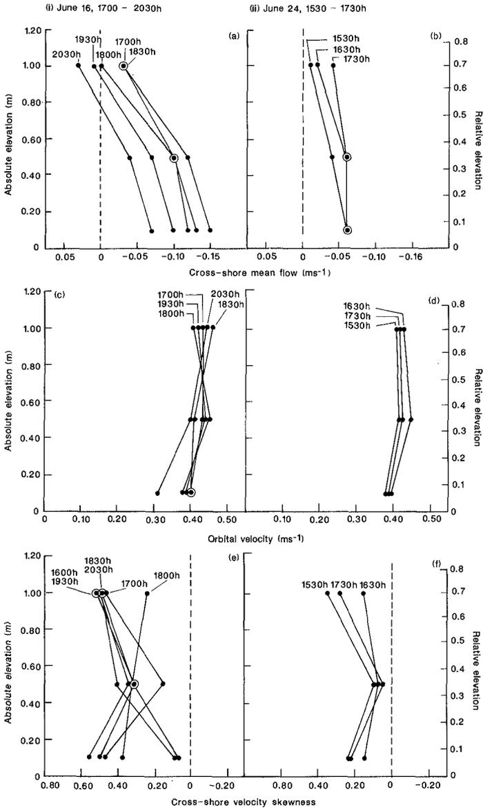
Figure 5. Vertical variation in the horizontal velocity field at 65 m offshore: i) 1700 - 2030 h on June 16; ii) 1500 - 1800 h on June 24; cross-shore mean velocity,  $\bar{u}$ , (a, b); cross-shore orbital velocity,  $u_s$ , (c, d); cross-shore velocity skewness,  $u_{sk}$ , (d, e). Note: positive values indicate onshore direction.
