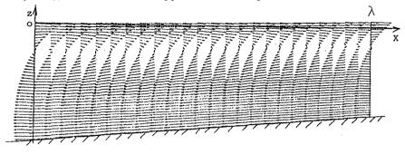
Fig.4 Test calculation of undertow velocity profile
