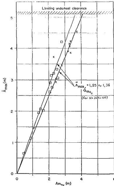
Figure 7. Maximum motion amplitude versus significant motion amplitude
