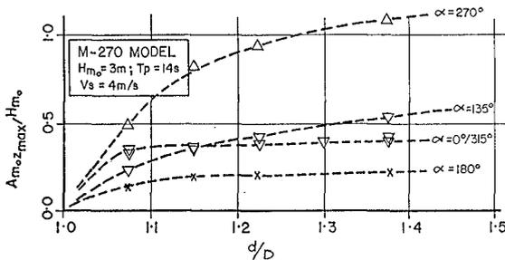
Figure 2. Maximum significant motion amplitude versus water depth
