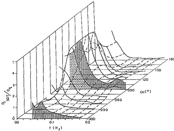
Figure 6. Motion amplitude response function for M270 Model
