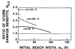
Figure 10. Ratio of Storm Damage Benefits, RSD, vs Initial Beach Width,  $w_0$ , and Additional Beach Width,  $\Delta w$ . RSD is Ratio of Storm Damage Benefits for Sand Which Spreads Out Immediately to Those for Which Sand Remains Where Placed.
