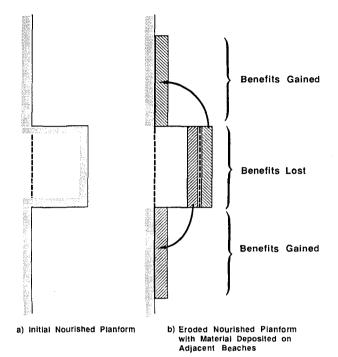
Figure 5. Schematic of Erosion of Nourished Area and Deposition in Project Adjacent Areas.
