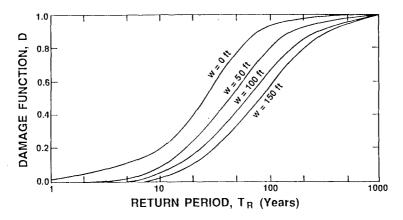
Figure 7. Hypothetical Proportional Storm Damage, D, as a Function of Storm Return Period,  $T_{\rm R}$ , and Beach Width, w.
