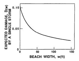
Figure 8. Expected Damage  $\bar{D}(w)$  Due to a Single Storm as a Function of Beach Width, w.
