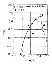
Fig. 10 Maximum scour depth vs. wave height in no-ripple regime.
