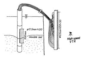
Fig. 2 Schematic diagram of a test pile with one hundred optical fibers and a high speed VTR.
