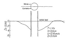
Fig. 5 Cross section of a scour hole in the longitudinal direction of the flume.
