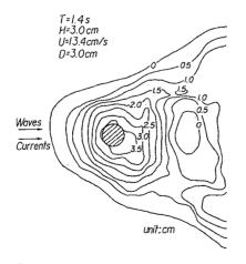
Fig. 4 Bottom topography of a typical scour hole.
