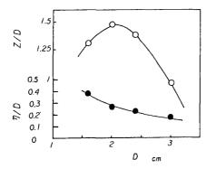
Fig. 12 Changes of scour depth and ripple height with a pile diameter.
