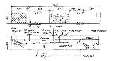
Fig. 1 Experimental apparatus and wave flume.
