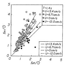
Fig. 8 Relationships between onshore and offshore radii of a scour hole.
