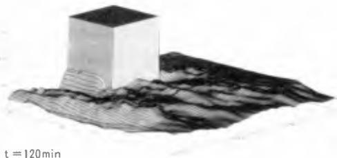
Fig.13 Bird's eye view of measured bottom change
