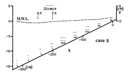
Fig.3 Distribution of the steady currents for Case 5.
