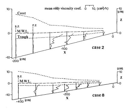
Fig.5 Distributions of the mean eddy viscosity coefficient for Cases 2 and 8.
