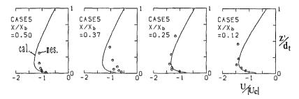
Fig.10 Comparisons between the measured and the calculated undertow profiles for Case 5.
