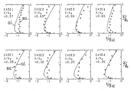
Fig.8 Comparisons between the measured and the calculated undertow profiles for the 1/20 slope.
