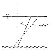
Fig.7 Assumed distributions of the mean Reynolds stress and the mean eddy viscosity coefficient. model. The constants in the model were investigated as follows.
