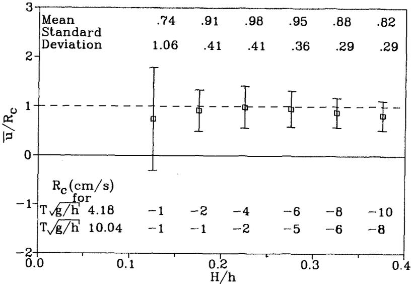
Figure 5: Mean and standard deviation of the normalized return flow vs. the relative wave height for all the runs. In the bottom of the figure the theoretical return flow is shown at each wave height for the 2.5 sec. and 6. sec. waves.
