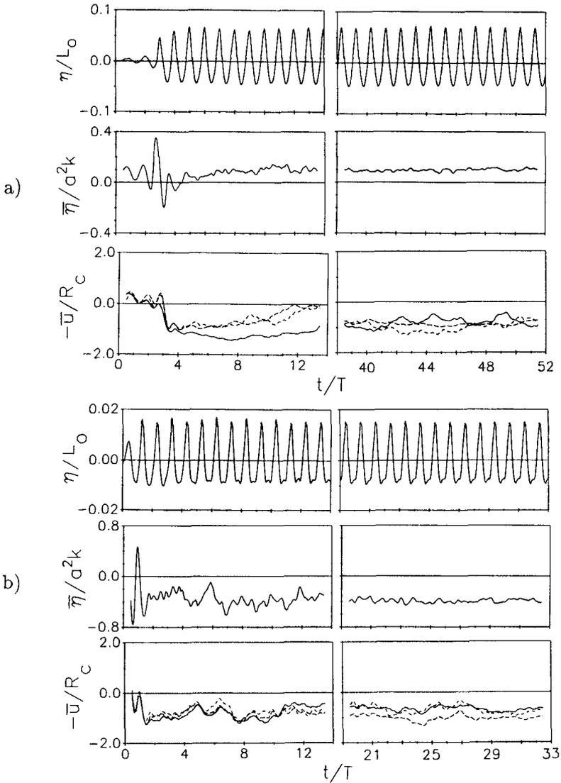
Figure 4: Nondimensional water surface profile, mean water surface, and return flow vs. time. Wave conditions: (a)  $T=2.5$  sec. ( $T\sqrt{g/h} = 4.18$ ),  $H=1.07$  m. ( $H/h = .304$ ); and (b)  $T=5.3$  sec. ( $T\sqrt{g/h} = 8.87$ ),  $H=1.07$  m. For  $-\bar{u}/R_c$  the various lines correspond to (—)  $z/h = -.74$ , (----)  $z/h = -.33$ , and (- - - -)  $z/h = -.32$ .
