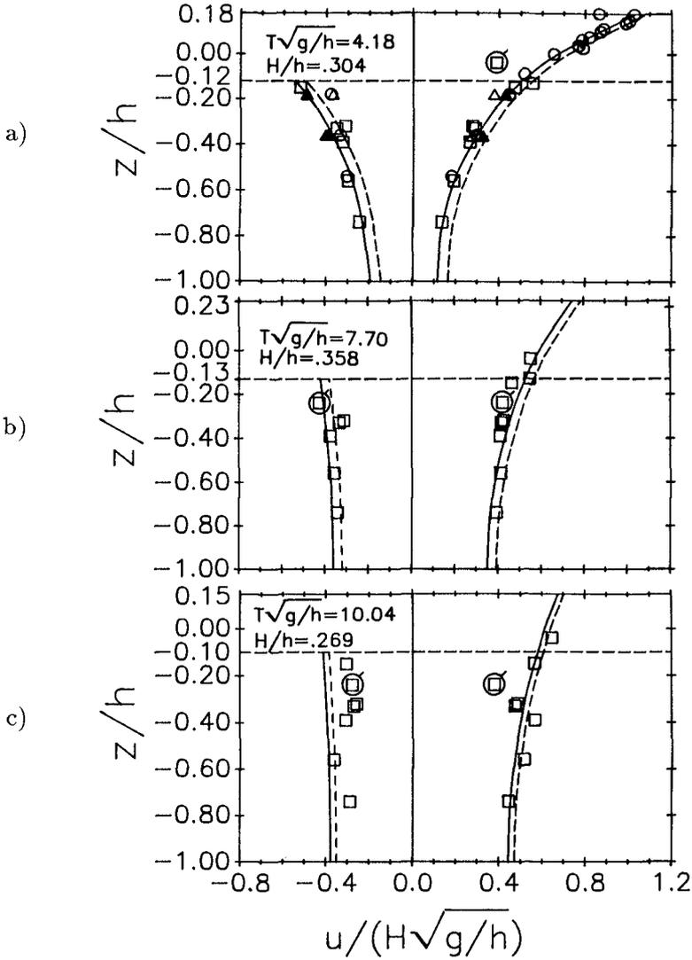
Figure 3: Nondimensional horizontal velocity under the wave crest and trough vs. relative depth. Figures 4a, b, and c show the results of Ramsden ( $\square$ ) electromagnetic current meters, (—) stream function theory, (---) stream function theory with return flow theory, and ( $\circ$ ) questionable measurements. Figure 4a also shows the measurements of Jensen (1978) ( $\circ$ ) propellor meter and Kobune (1978) ( $\blacktriangle$ ) hot film anemometer, ( $\triangle$ ) propellor meter.
