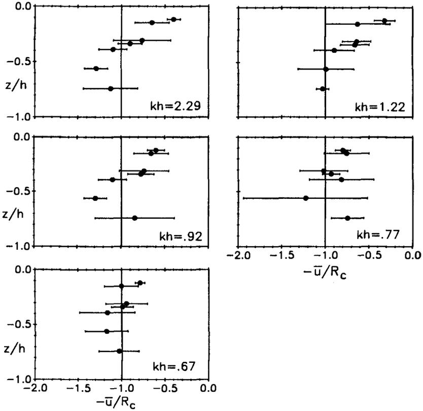
Figure 6: Mean and standard deviation of the nondimensional return flow, averaged over the wave height, vs. the relative depth for each wave period.
