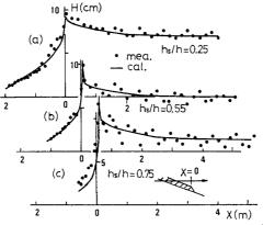
Fig.8 Wave height distributions on the reef(Hi/h=0.9)
