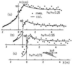
Fig.9 Wave height distributions on the reef(Hi/h=0.75)
