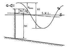
Fig.2 Definition sketch of wave overtopping
