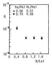
Fig.13 Non-dimensional wave overtopping rate vs. nondimensional length of artificial reef
