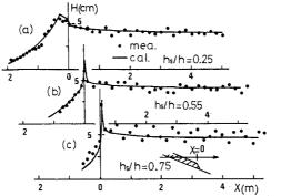
Fig.7 Wave height distributions on the reef(Hi/h=0.5)
