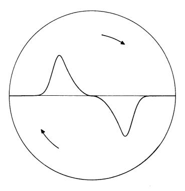
$$\begin{split} V_{r} &= 0 & \text{with:} \\ V_{\theta} &= C_{5} \left[ \frac{r}{R_{1}} \right]^{N} & \text{for } r < R_{1} & C_{5} = 0.9 \text{ m/s} \\ & C_{5} = 0.9 \text{ m/s} \\ & C_{6} = 1.0 \text{ m/s} \\ & R_{1} = 900 \text{ m} \\ & R_{2} = 1000 \text{ m} \\ & R_{2} = 1000 \text{ m} \\ & R_{3} = 300 \text{ m} \\ & N = 2 \end{split}$$
