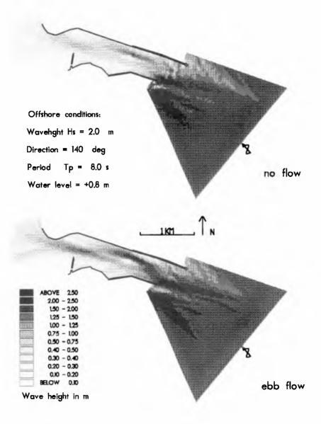
Figure 6 Malamocco inlet to the Venice lagoon area; effect of an ambient current field on the wave height distribution
