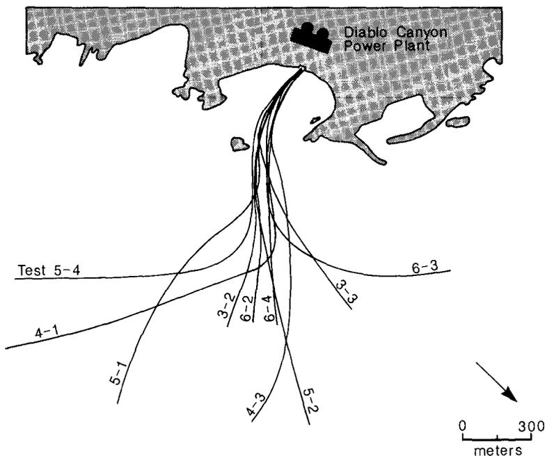
**Figure 6. Offshore Plume Centerline Trajectories**
