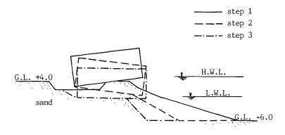
Figure 4. Procedure of caisson floating out -- Sit-to-Float. Steps: 1) dredging and washing out sand around caisson bottom; 2) caisson lowing down at L.W.L.(lowest water level) on its own weight; 3) caisson floating out at H.W.L.(highest water level)
