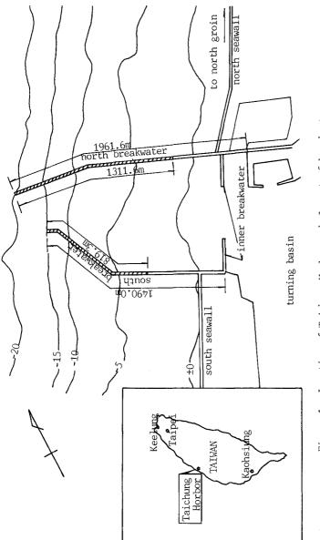
Figure 1. Location of Taichung Harbor and Layout of breakwater, shadow part indicates composite section
