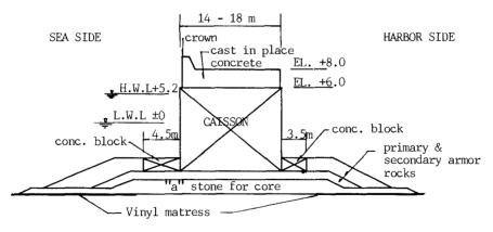
Figure 2. Typical cross section of composite type breakwater at Taichung Harbor
