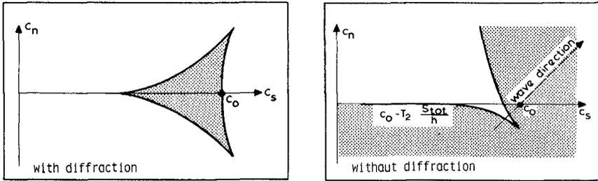
Fig. 3 Influence of wave diffraction on bottom celerities
