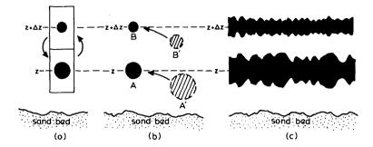
Fig. 1 Sediment exchange due to diffusion (a), motion of sediment concentration under waves (b), and time-averaged local concentrations at levels z and  $z+\Delta z$  (c).
