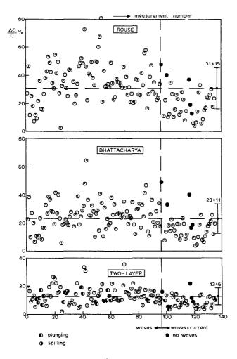
Fig. 3 Results for AC/C for the various models
