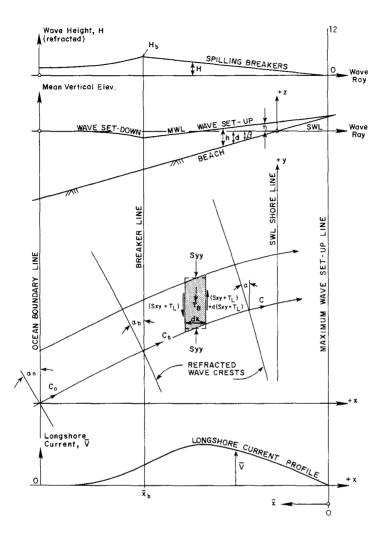
Figure 1. Schematic of surf zone (from Basco, 1982)
