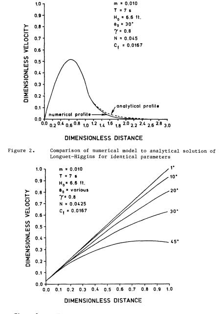
Figure 3. Numerical model results for large angle effects without lateral mixing
