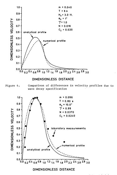
Figure 5. Comparison of predicted velocity profile with laboratory measurements of Mizuguchi et al. (1978 Case 3)
