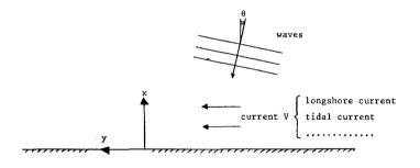
Fig. 1 - Combination of a current and a wave field; θ = angle of incidence, x = coordinate normal to the coast, y = coordinate in longshore direction.
