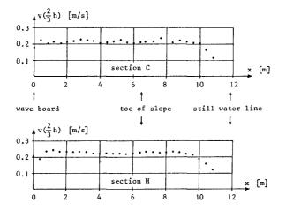
Fig. 6 - Distribution of mean current velocity v at a height of z = 2h/3 in sections C and H in exp. 1.01 (current alone).
