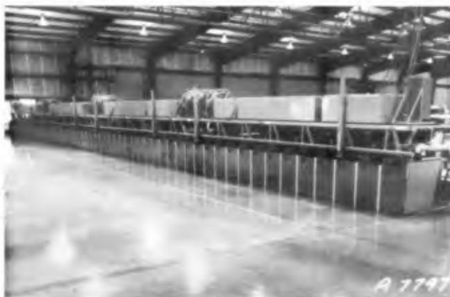
Figure 3. The Directional Spectral Wave Generator
