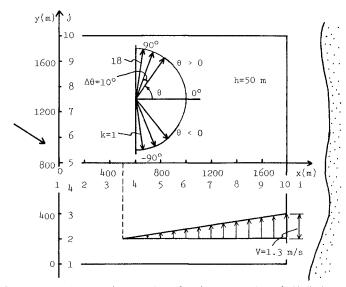
Fig.2 Computation region, water depth, current and division of wave direction
