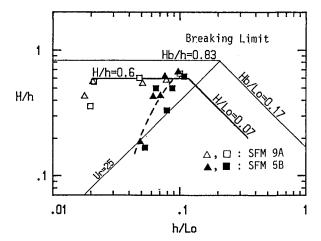
Fig. 11 Application Ranges of the SFM 9A and SFM 5B Theories.
