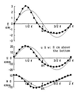
Fig. 3 Comparisons between Measured and Predicted Wave Form and Velocities for ST 1 and ST 5 Theories.
