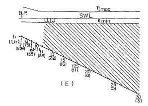
Fig. 7 Validity Limit for Horizontal Velocity of ST 5 Theory (Exp. 2-1)
