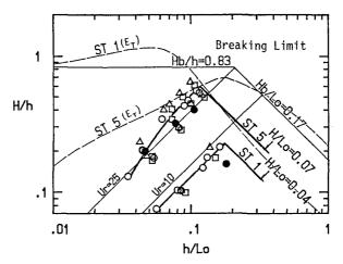
Fig. 9 Application Ranges of ST 1 and ST 5 Theories.  $\circ$  • : the wave surface elevation,  $\circ$  • : near-bottom horizontal velocity,  $\circ$  • : horizontal velocity below the trough. —— : isoline of  $E_m = 0.10$  by Isobe (1986)
