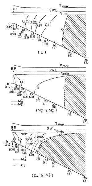
Fig. 6 Validity Limit for Horizontal Velocity of ST 1 Theory (Exp.2-1).
