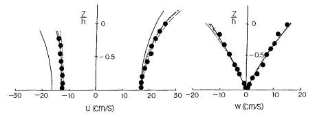
Fig. 5 Vertical Distributions of Water Particle Velocities under Crest and Trough (Exp. 2-1, Ur = 22).
