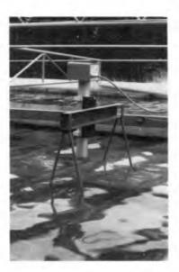
Fig.6 Servo-Type Wave Gage
