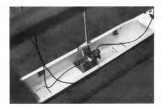
(a) Potentio-Meters Installed at C.G.
