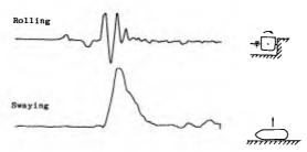
Fig.9 Time-Histories of Ship Waves and Vessel Motions
