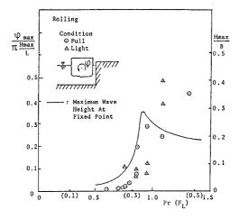
Fig.14 Maximum Rolling Motions of Moored Vessel
