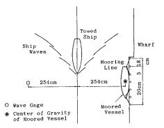
Fig.5 Model Set-Up
