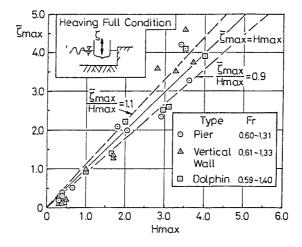
Fig.15 Maximum Heaving Motion of Moored Vessel
