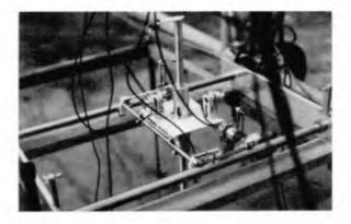
(b) Potentio-Meters Equipped on Upper Carriage Fig.8 Measurement of Vessel Motion
