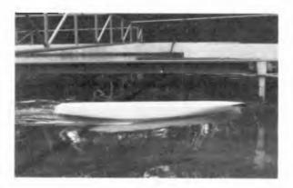
Fig.1 Model Ship Towed by Carriage
