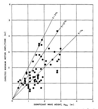
Figure 2. Maximum vertical ship motions at Richards Bay harbour
