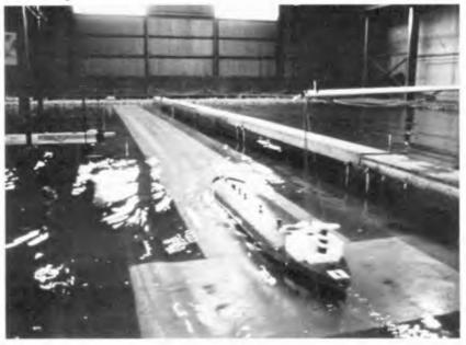
Figure 15. Model test run with 90° wave approach
