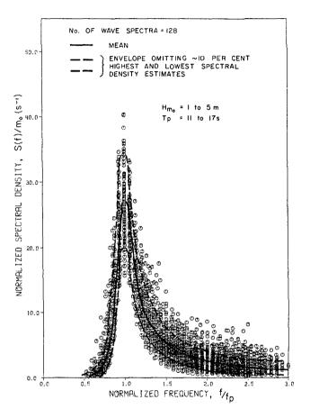
Figure 16. Normalized Richards Bay wave spectra
