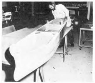
Figure 3. Mould for construction of glass fibre model hull
