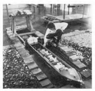
Figure 4. Distribution of lead weights for proper loading
