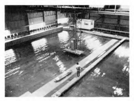
Figure 6. Model test basin with Seasim irregular wavemakers
