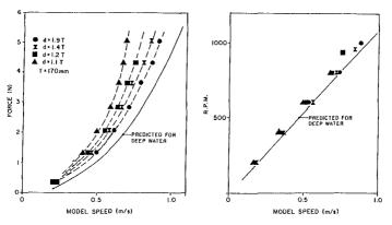
Figure 12. Model towing resistance and speed
