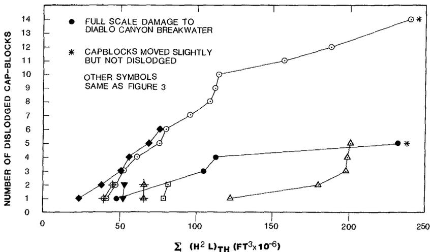
Figure 4. Cap-block Displacement Versus Cumulative Wave Energy. Based on  $(H^2L)_{TH}$  of 230,000 ft<sup>3</sup>. Each Tribar weighs 21.6 tons.
