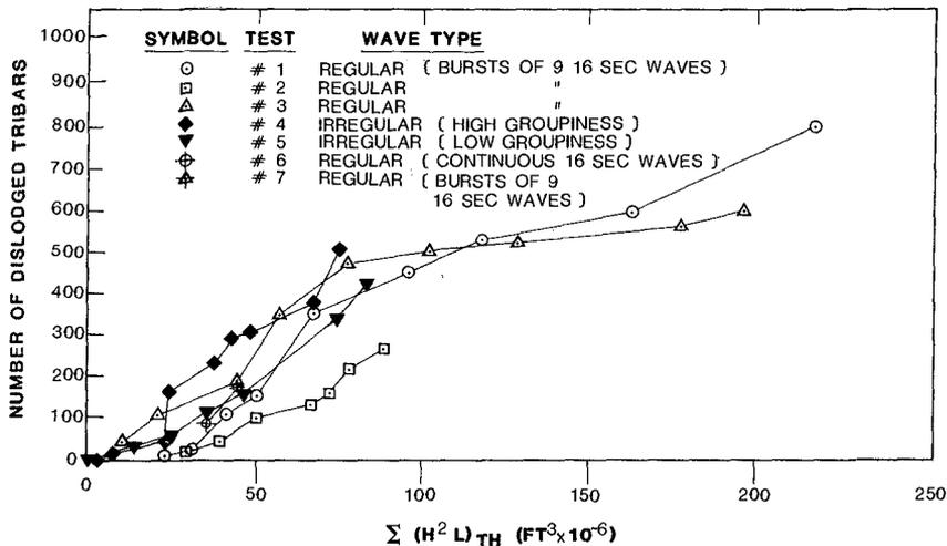
Figure 3. Tribar Displacement Versus Cumulative Wave Energy. Based on  $(H^2L)_{TH}$  of 230,000 ft<sup>3</sup>. Each Tribar Weighs 21.6 tons.
