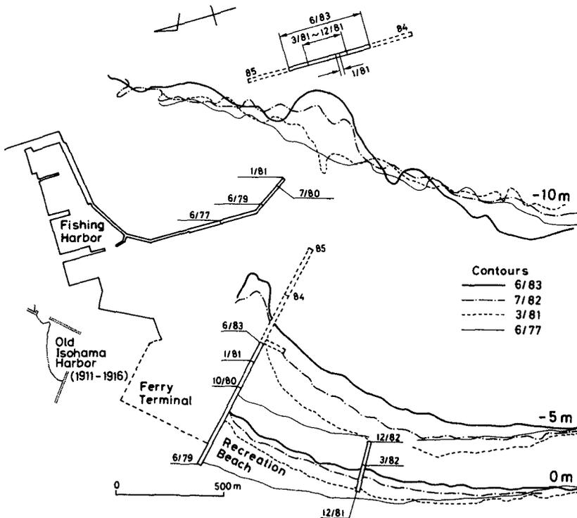
Fig. 1 Construction and contour change at Oarai.
