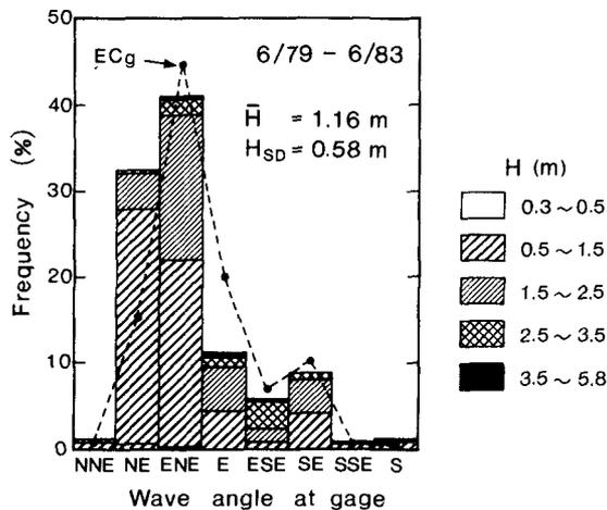
Fig. 3 Wave height, direction, and energy flux ( $EC_g$ ).
