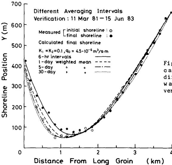
Fig. 10 Shoreline change calculated by using different time-averaged wave inputs for the verification period.
