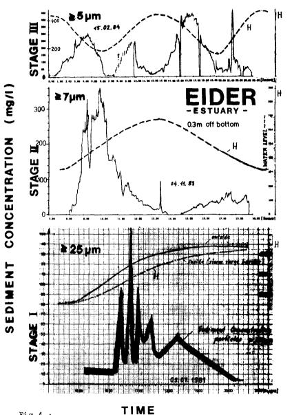
Fig.4 : **IIME** Simultaneous records of suspended sediment concentration and water level (tidal curve)
