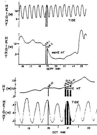
Figure 3. Environmental conditions. The significant wave height was measured by a waverider buoy in 20 m of water. The tides are semidiurnal and have a range of 0.75 to 1.3 meters.
