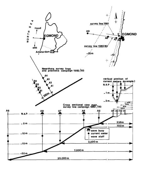
Fig. 1 Location and measurement set-up
