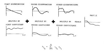
Figure 9: Eigenfunction Decomposition of the Profiles
