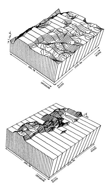
Figure 7: Location of Erosion and Accretion due to October Storm. (Straightened Shoreline, Exaggerated Scale)
