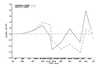
Figure 4: Incremental and Cumulative Change in Volume of Beach Sand over the Survey Area. (Survey Dates Denoted by Vertical Bars on Abscissa.)
