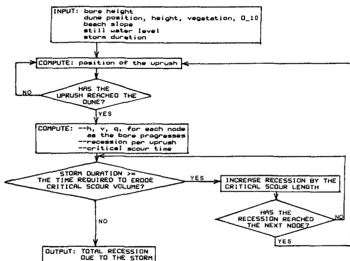
FIGURE 3. Flow chart of the uprush/dune erosion model.
