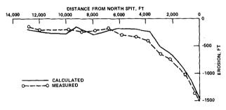
Figure 6. COMPARISON OF CALCULATED AND MEASURED SHORE-NORMAL EROSION OREGON INLET, NORTH CAROLINA (BODIE ISLAND, 1962 ASH WEDNESDAY STORM)
