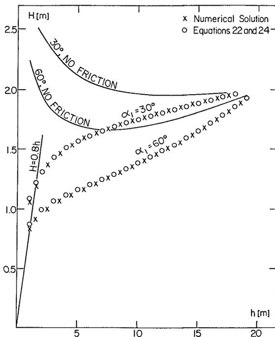
Figure 7: Comparison between the explicit solution (equations 22 and 24) and a numerical solution. The shown example corresponds to  $T = 8s$ ,  $f_e = 0.1$  and a beach profile given by  $h = 0.1(x_o - x)^{2/3}$ .
