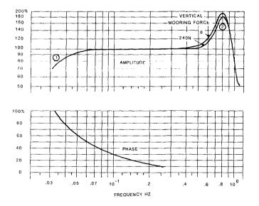
FIGURE 4: WAVERIDER TRANSFERFUNCTIONS (WAVERIDER MANUAL)
